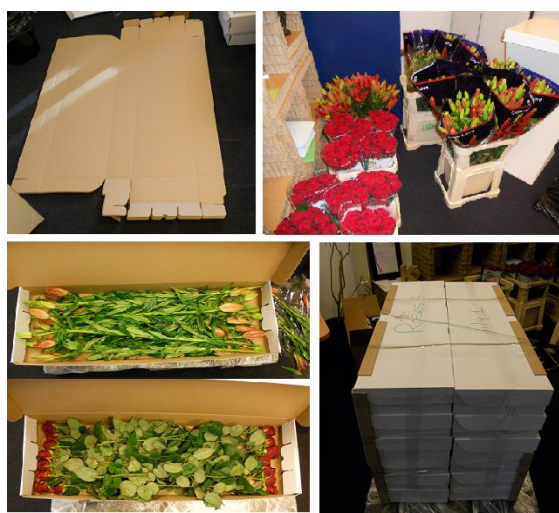
Transport tests with boxes coated with an active substance to enhance flowers' vase life.
